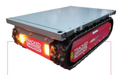
The 1200 series from Tracked Carriers is the ideal all-round carrier. At just 750mm wide the 1200 R and 1200 PRO models can fit through most doorways, and with a substantial 1,200kg maximum capacity the uses are endless.
